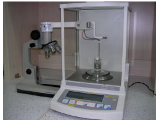
Fig. 4: The set up during a measurement. The arm enters the housing of the precision balance while the body of microscope remains outside. The mercury cup is shown on the balance. We move the cage and the stick and the needle up and down by using gross and fine adjustment knobs on the microscope
