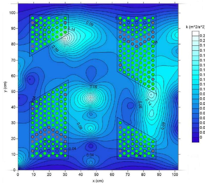
**Figure 7.** Turbulent kinetic energy,  $k$ , distribution in x-y plane at the central flow depth for  $d/h=0.92$ .
