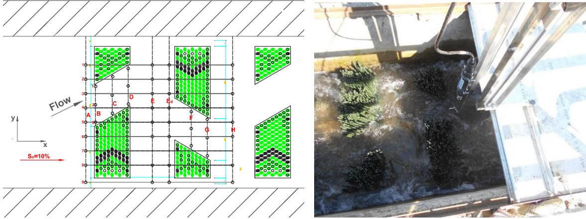
**Figure 3.** Top view of the brush fishway and the velocity measurement grid.
