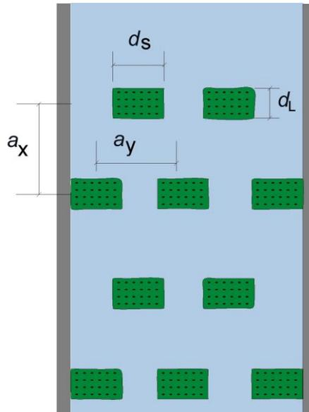
**Figure 1.** Drawing of a brush fish pass. Adopted from DWA (2014).
