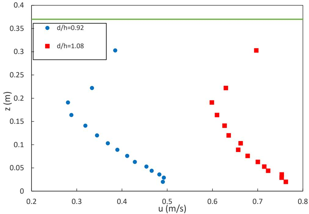
**Figure 5.** Vertical velocity profiles for different bristle relative submergences.
