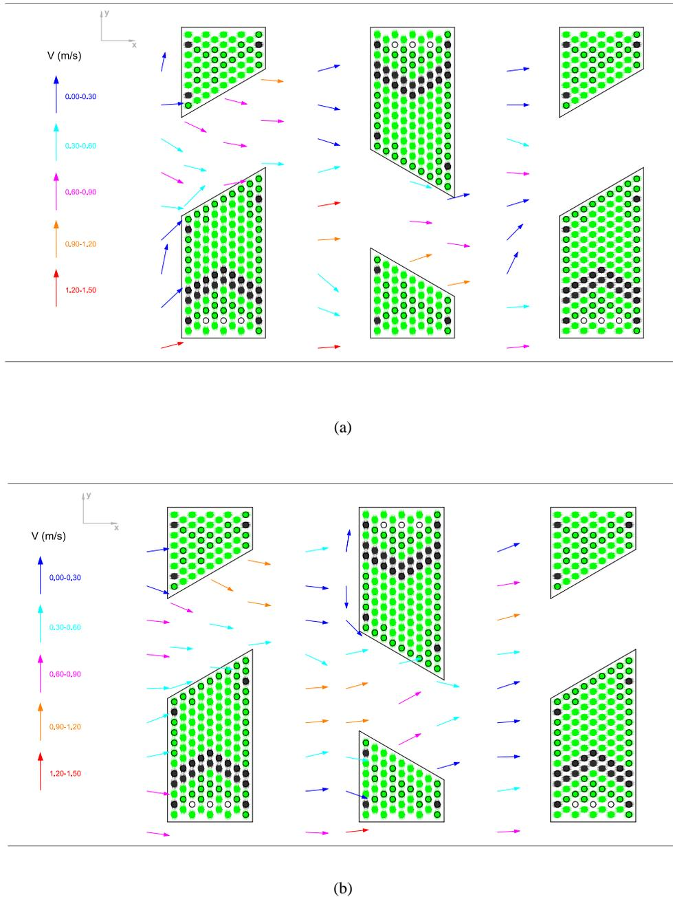
**Figure 4.** Flow field in the horizontal plane for  $d/h=0.92$  at (a) channel bottom and (b) central flow depth.
