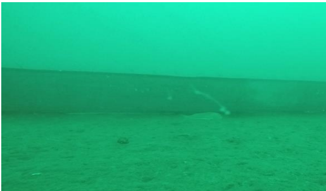
Figure 3. Standing of the cloth tarpaulin mounted nets underwater.
