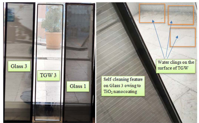
Figure 23. Visual quality of Glass 1 and Glass 3 in comparison with commercial air filled triple glazed window (TGW) and self-cleaning feature of Glass 3 through water spray test.
