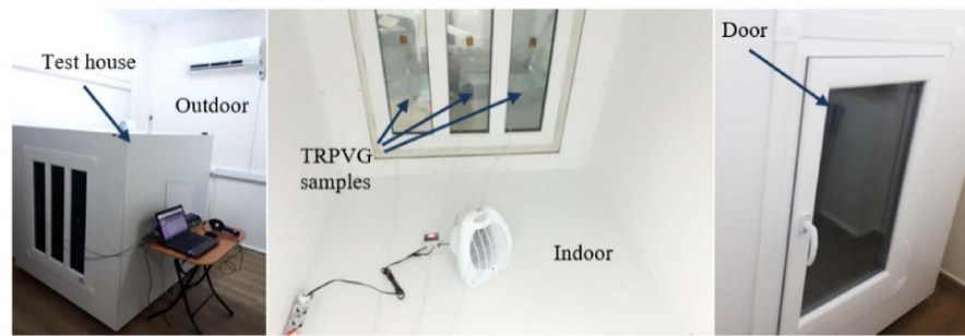
Figure 4. Test house used for acoustic tests of TRPVG.
