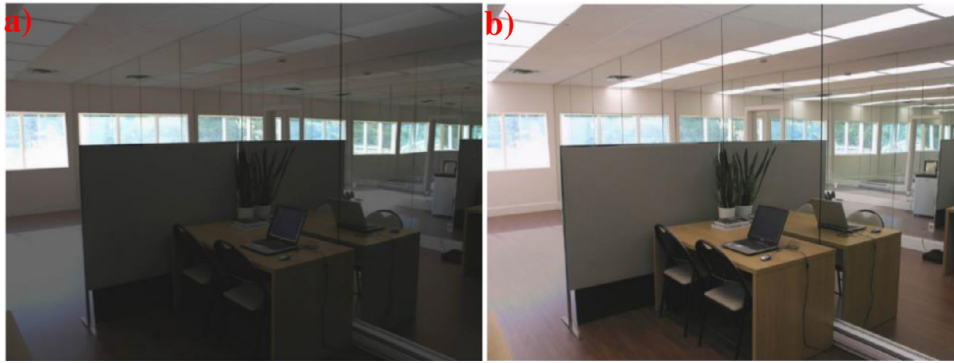
Fig. 4. Workplace illuminated by typical daylighting through (a) the window only and (b) the solar canopy system with window [44].
