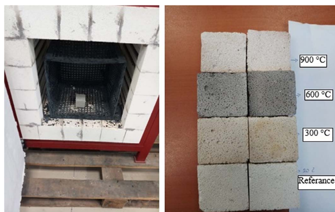
Figure 7. Variations in mortar samples after exposure to high temperature.
