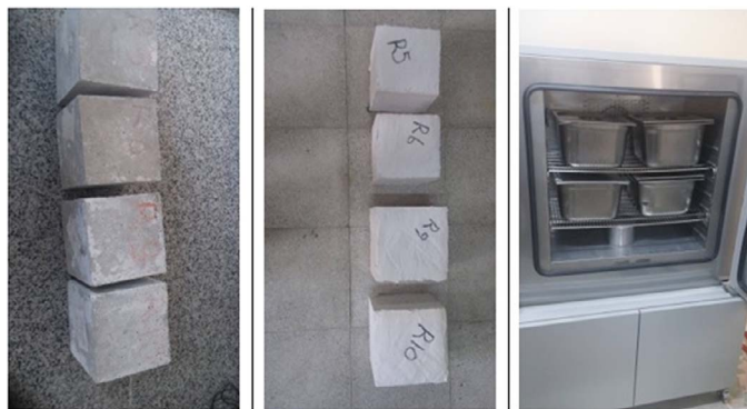
Figure 6. Changes in the mortar-coated concrete sample before and after the frost test.
