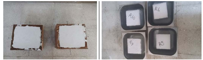
Figure 5. Samples of mortar-coated concrete prepared before the frost test.
