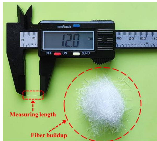
Figure 3. Physical view of the polypropylene fiber used.
