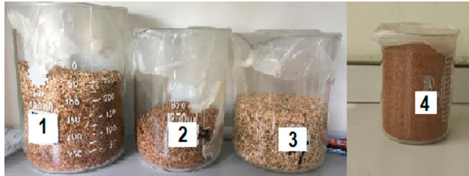
Figure 1. The appearance of biomass samples and combinations (1—mixed biomass samples 2—walnut shell 3—tea bush 4—pine cone).
