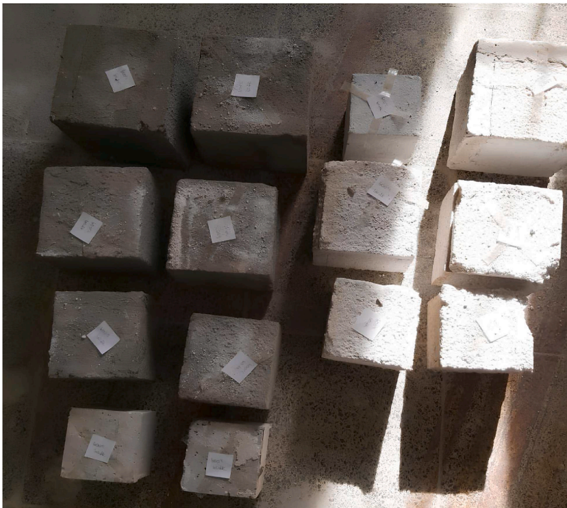
Fig. 7. Samples, both with and without plaster, which is exposed to a temperature of 450 °C for 60-min.
