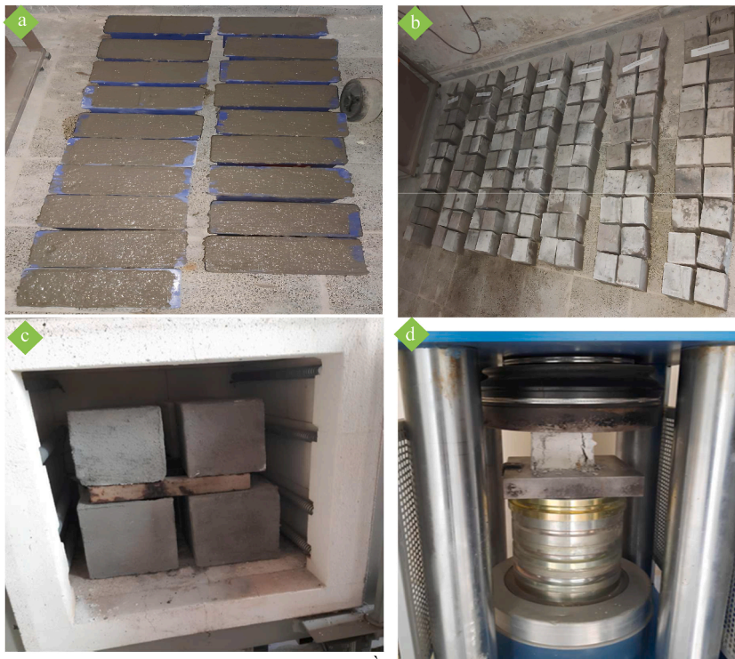
Fig. 1. a. The concrete generated by pouring the prepped mortar into the mould, b. The phase where samples are being plastered, c. The situation in which samples are placed inside an oven and exposed to heat, d. The act of subjecting the samples to CS testing.
