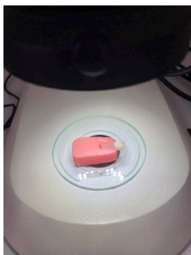
Fig. 4. Carrier mechanism prepared from autopolymerized acrylic resin.
