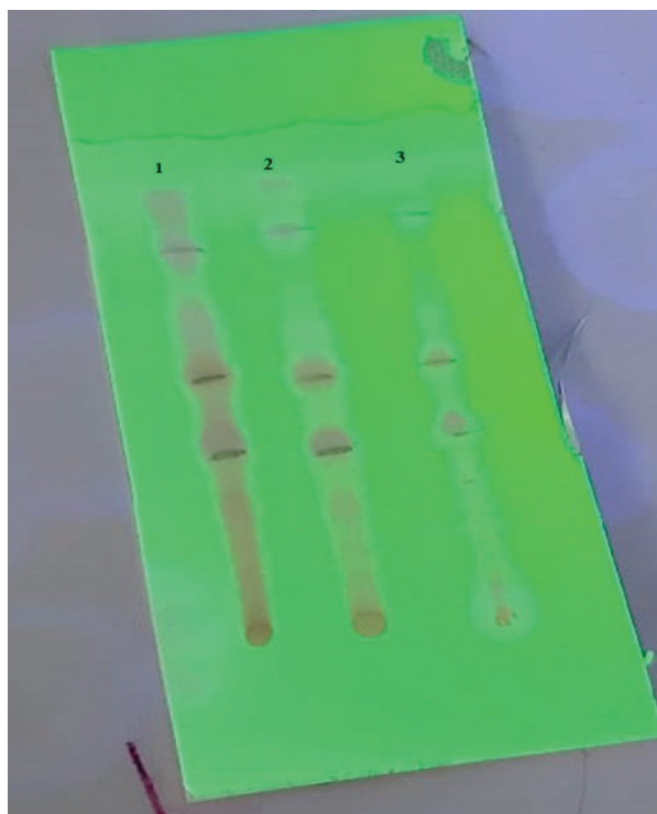
Figure 1. TLC image of samples. Lines as 1,2,3, Represents ethanol propolis extract, Residue and Water Soluble Fraction respectively.
