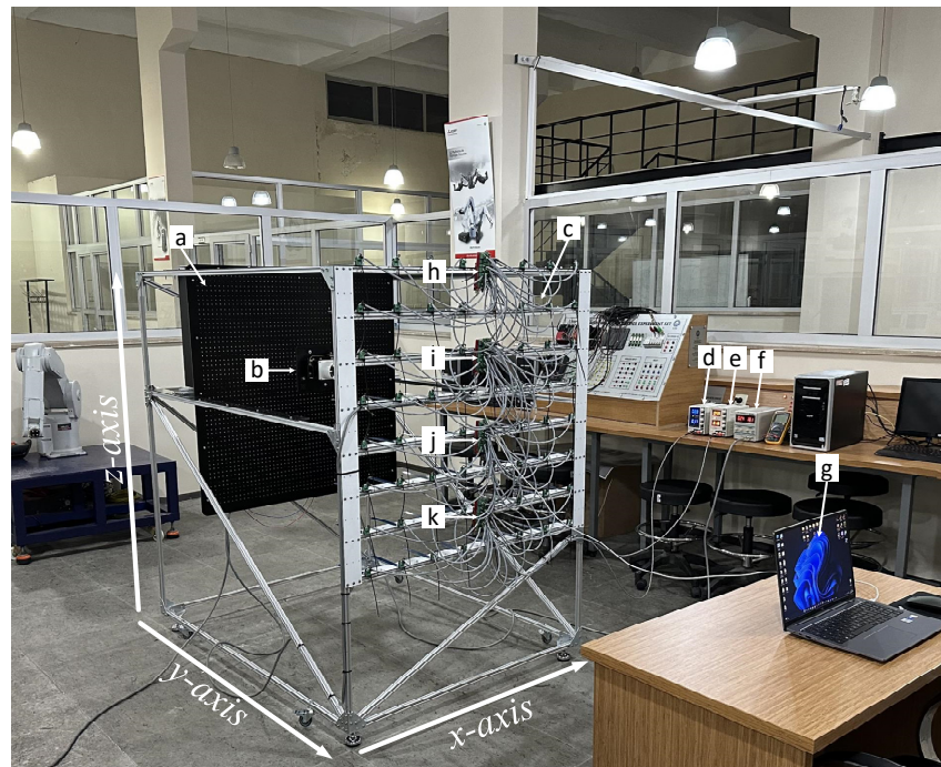
Figure 9. General view of the temperature measurement system: (a) measurement plate; (b) fan heater; (c) 8 \times 8 sensor grid; (d) power supply 1; (e) power supply 2; (f) power supply 3; (g) computer (h) LCU1; (i) CCU; (j) LCU2; (k) LCU3.
